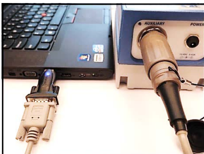
2b. Serial Cable (Part # 720A3101) to Serial-to-USB adaptor (Part # 714A7001) to USB port
