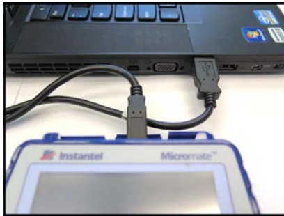
Micromate's PC port to Computer USB
