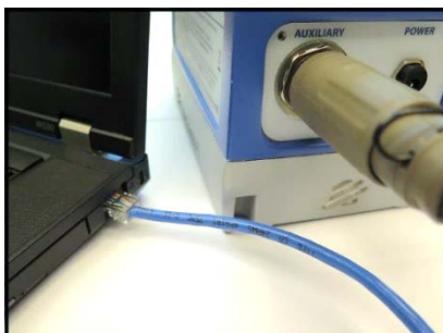
2c. Ethernet cable (Part # 720A4101) to Ethernet port
