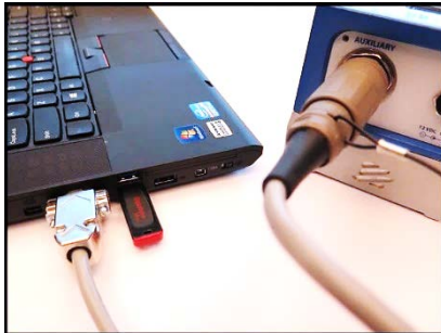
2a. Serial Cable (Part # 720A3401) to Serial port
