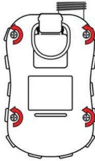
5. Hold the ToxiRAE Pro down and separate the rear cover from the front by pulling from the top and tilting it open without disconnecting the ribbon cable connecting the two halves.
